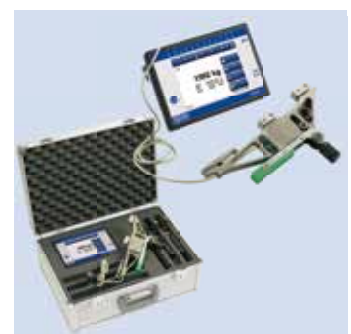
Fig. 38: Simultaneous measurement of rope tensile force
